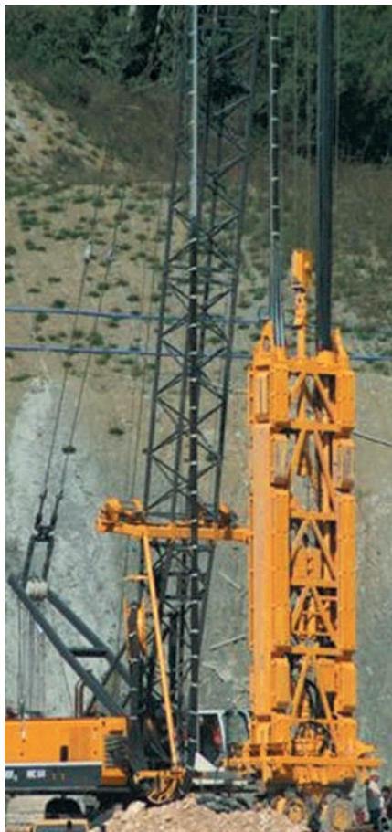
Fräse Trench cutter
