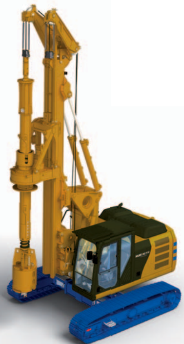
Low head drill configuration
