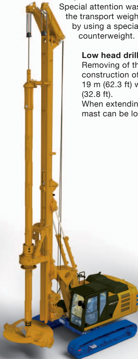
Rathole drill configuration
