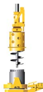
Cased Kelly drilling (installation with oscillator)
