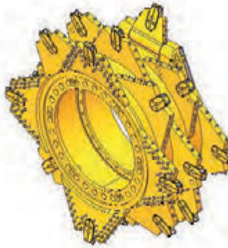
Four tooth holders in one row of teeth
