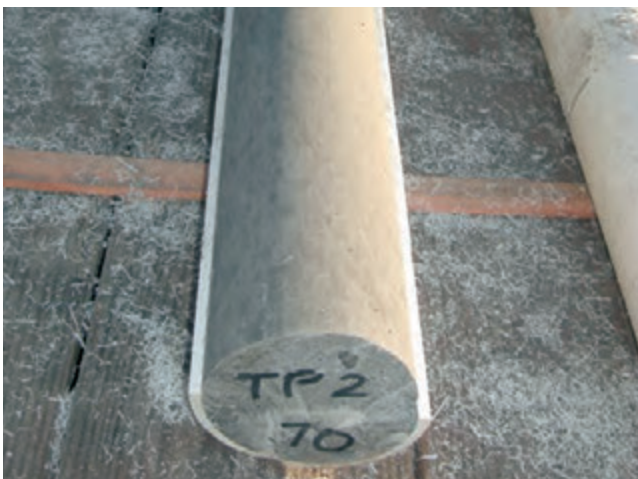
Cut-open inner plastic tube with hardened core
