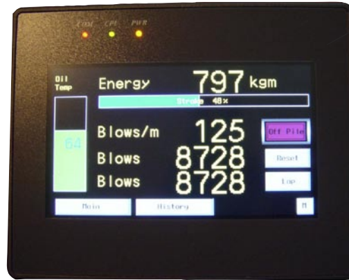
INTERFACE SCREEN MOUNTED ON POWER PACK
