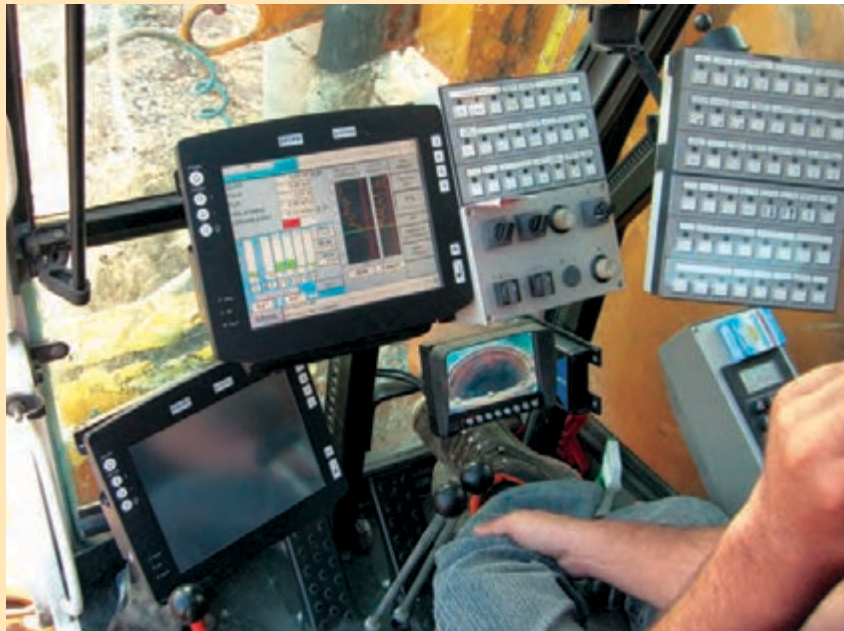
Touchscreen with display of essential parameters in automatic drilling mode.
