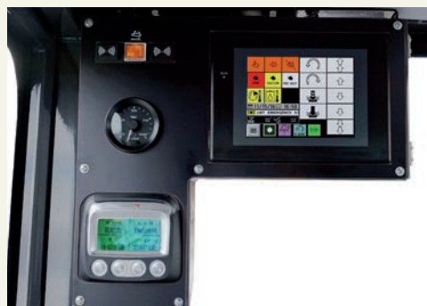
The monitoring system incorporates gauges in the cabin, allowing the operator a quick visual of engine temperature, hydraulic oil temperature and fluid levels.
