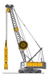
Hydraulic grab DHG with hose drum system HDSG 50/HDSG 80
