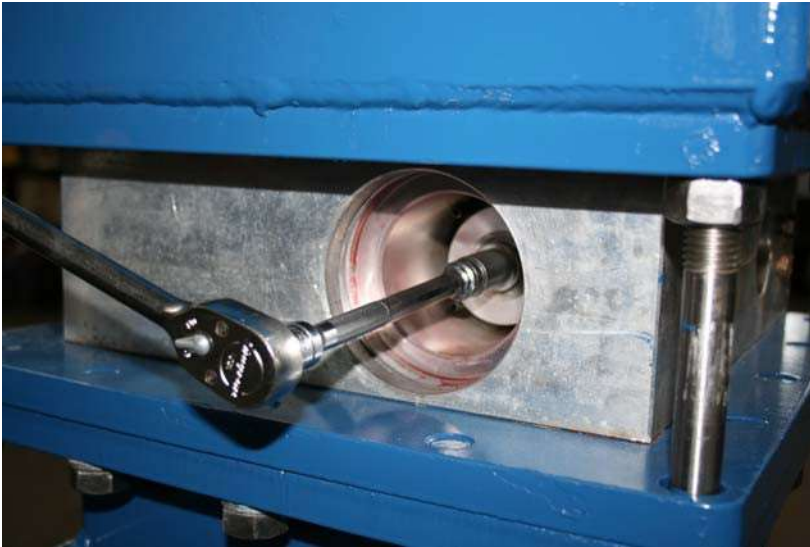
A 3/4-inch socket with extension is used on the nut at the spring end.
