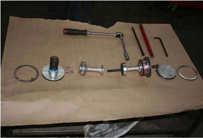
The complete valve spool (with the spring being held in place with RTV silicon).
