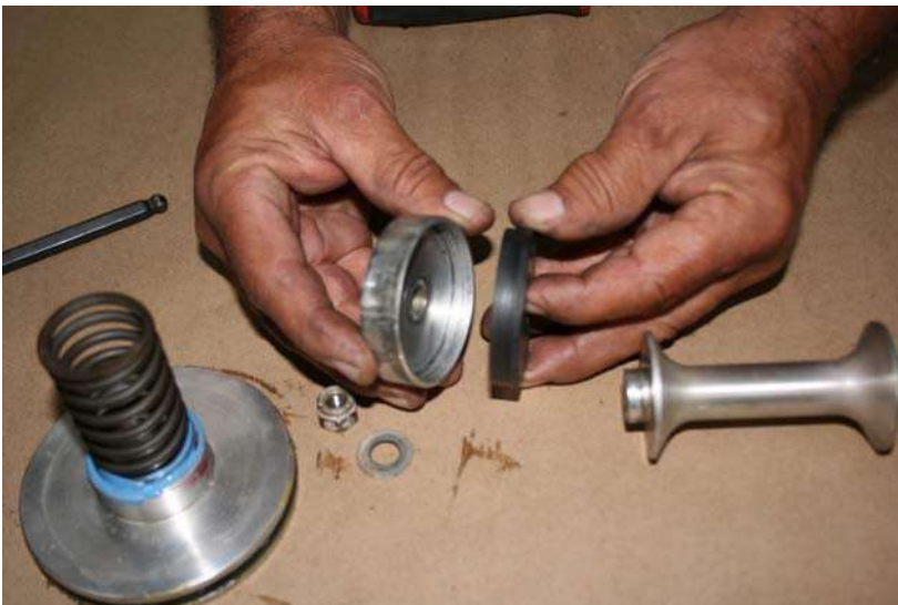
The seal is easily removed, and can often be turned around one time before it needs to be replaced.
