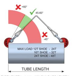
1/2 TUBE LENGTH x 1.414 = MIN SLING LEG LENGTH
