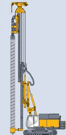
VdW Vor-der Wand Bohren Front-Of-Wall drilling
