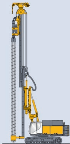
VdW Vor-der Wand Bohren Front-Of-Wall drilling
