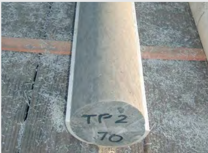
Cut-open inner plastic tube with hardened core
