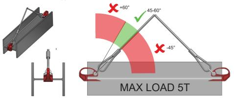
Lifting Angle Range 45-60° Sling legs must be of equal length. Angles less than 45° could result in an over loading of the equipment.
