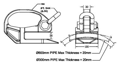
Lifting pipe using the SHS-908 Steel Pipe Shoe increases the range of steel pipe that can be handled and also the capacity
