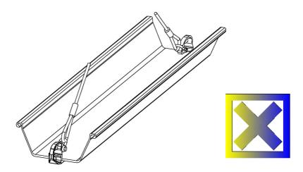
This is the correct method for lifting a pair of LX piles with two pairs of 900 shoes. Note the pairs of slings are of different lengths to ensure the piles are lifted uniformly.
