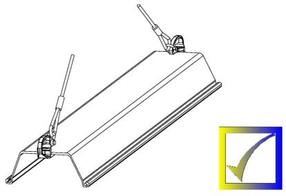
This is the incorrect method for lifting a LX pile with one pair of 900 shoes.
