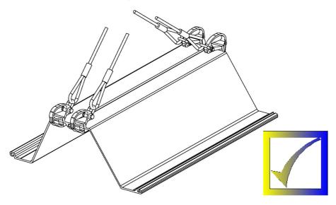
This is the incorrect method for lifting a pair of AZ piles with two pairs of 900 shoes.
